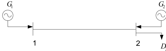
Figure 33: One Line Diagram of a Two-Bus System [43]
